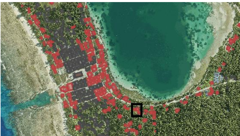
Figure 11: Location of Vaitupu Medical Clinic and buildings currently exposed by 1% AEP storm surge. The red highlights buildings that are exposed to hazards present day. (Source: Tuvalu Coastal Adaptation Project.)
